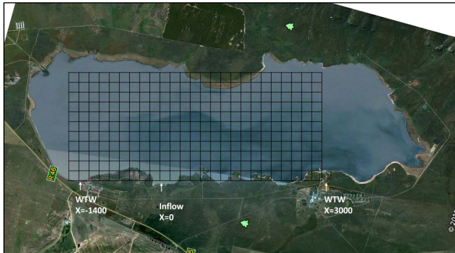
Figure 4: Illustration of the matrix that was set up to estimate the dispersion of bacteria in the transfer water.
