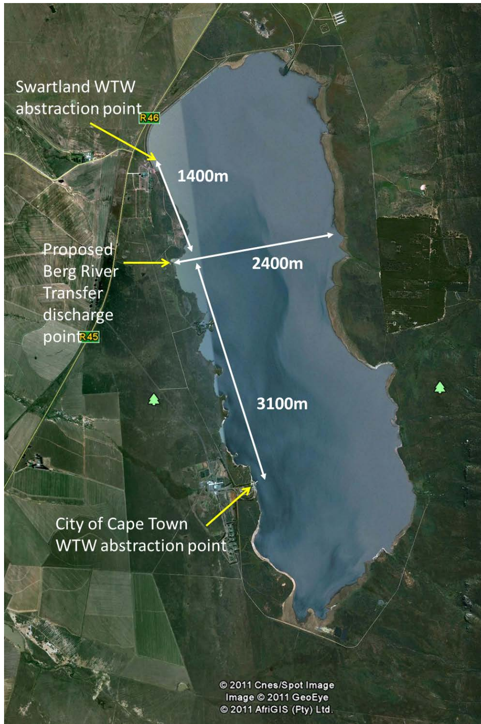
Figure 3: Image of Voëlvlei Dam showing the proposed location of the discharge point and approximate distances to the two WTW abstraction points.
